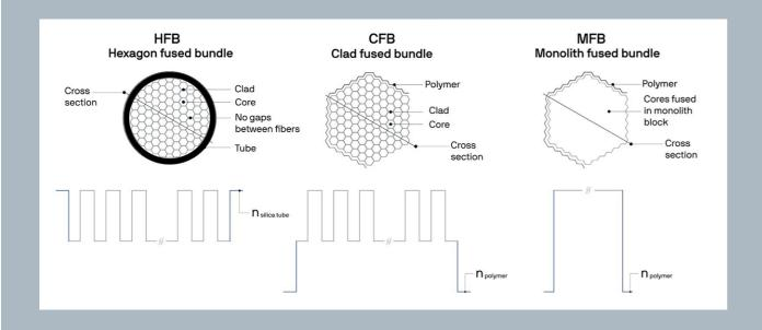
The upper row picture schematically explains the differences of different fused end fiber bundle technologies. In contrast, the bottom row shows RIPs of corresponding fiber bundle cross-sections. The main difference between conventional HFB and the new fused end fiber bundle technologies CFB and MFB is the absence of the silica tube.
