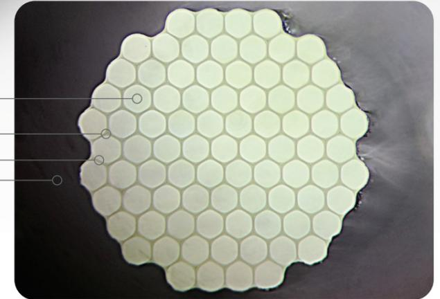
During fusing process fibers change shape to hexagonal (a) and are packet together in honeycomb structure with no free spaces in-between fibers (b), surrounding fibers are minimally defected (c) and fused end is surrounded by air or polymer (d).
