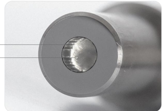
During fusing process silica fiber cores create monolith structure in length ~2cm (a), while in a dept is possible to see silhouettes of individual fibers (b).
