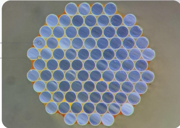
Individual fiber consists from synthetic silica core and F-doped silica reflecting cladding (a) and lost areas in-between fibers are filled with epoxy (b).
