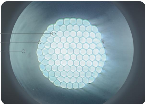
Fibers are pressed together with silica tube (c). Fibers change shape to hexagonal and are packet together in honeycomb structure (a), while surrounding fibers are defected and active end of bundle deviates from circular shape (b).
